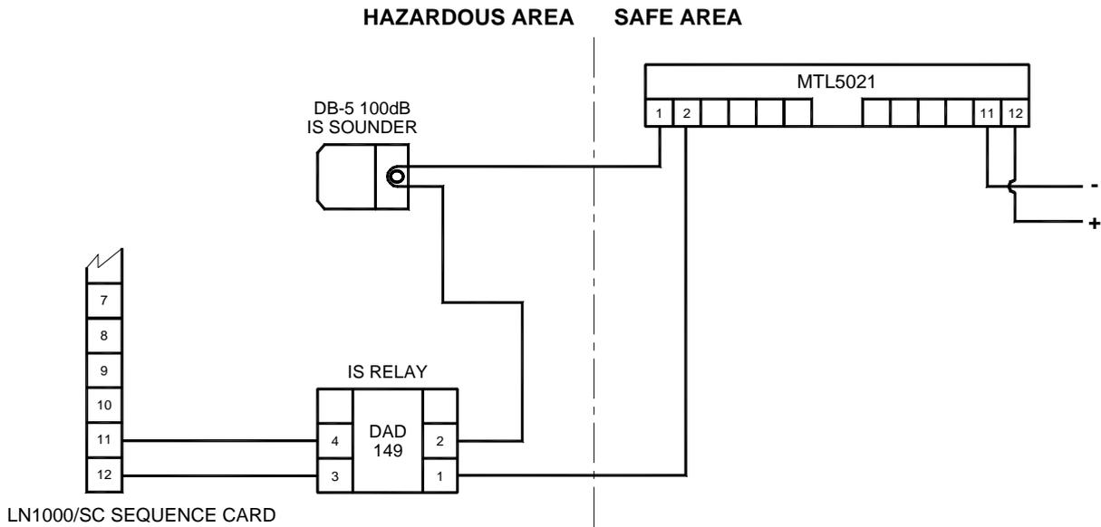
**Connections to sounder using hazardous area mounted IS relay (Figure 13.2)**
