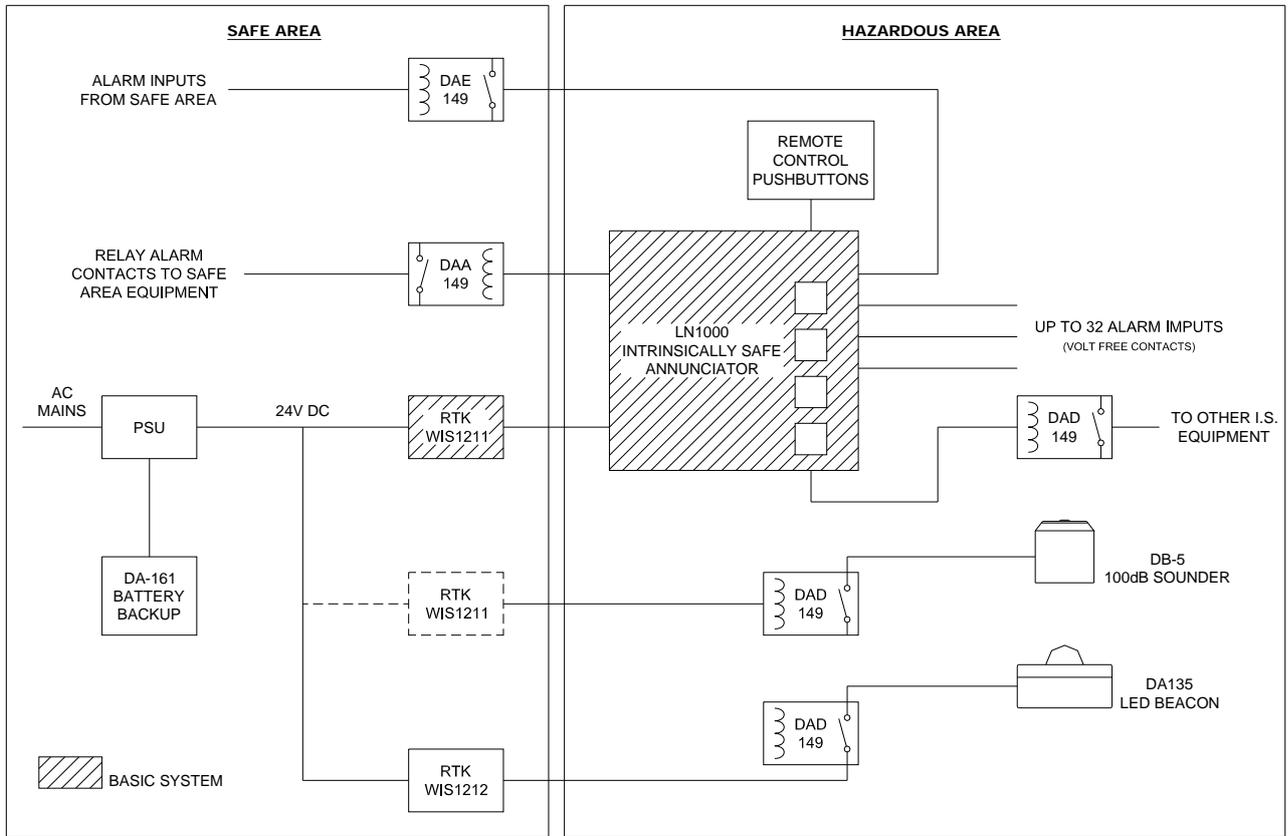
**Standard system configuration showing ancillary components (Figure 2.1)**
