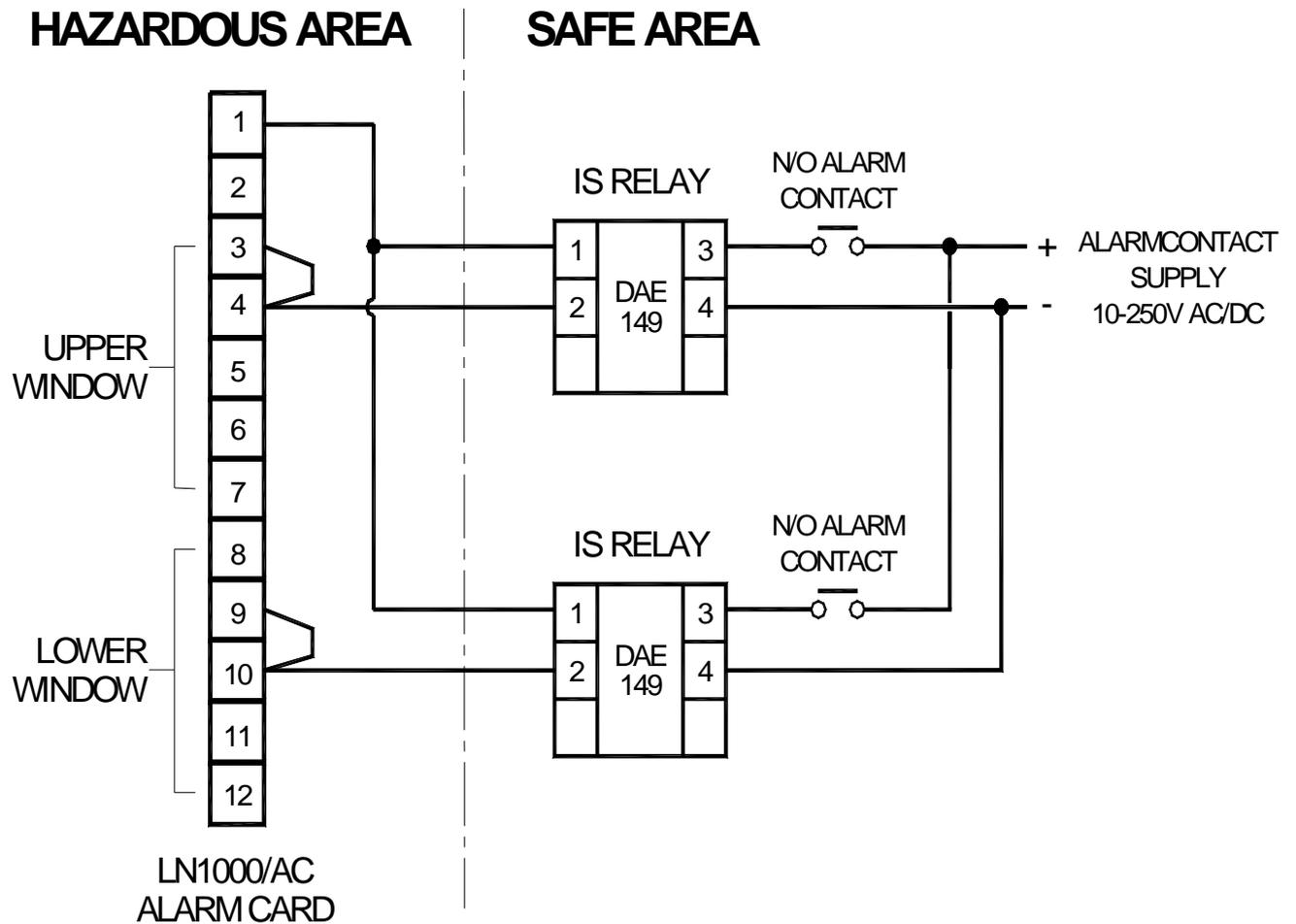
*Alarm ways with normally open contacts mounted in the safe area (Figure 12.4)*
