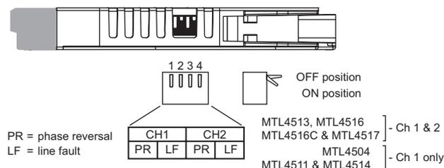
Record the settings of these switches for the module under test so that the condition can be restored following completion of the tests.
