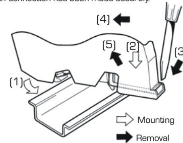
Fig. 1 - Mounting/removing a SLP unit
