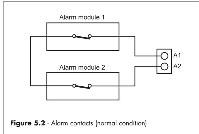
Figure 5.2 - Alarm contacts (normal condition)
