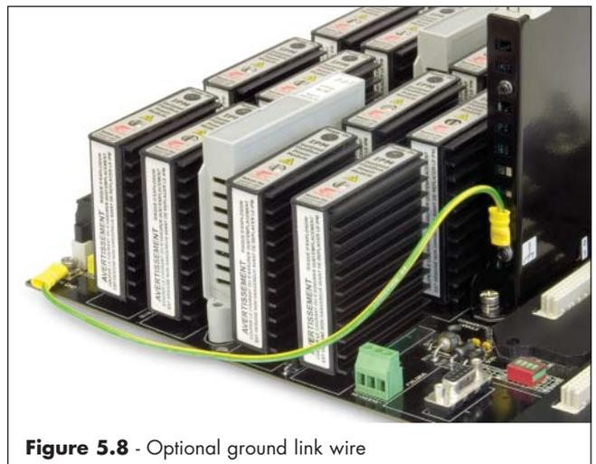
Figure 5.8 - Optional ground link wire
