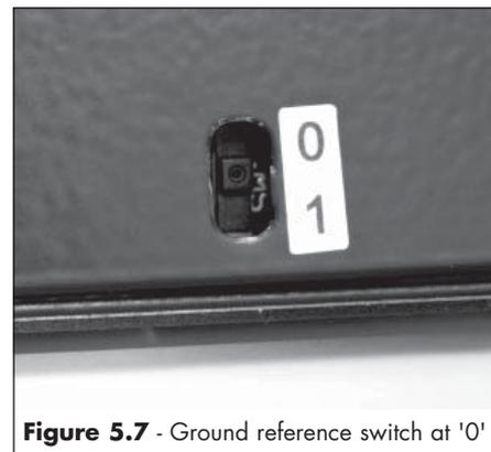
Figure 5.7 - Ground reference switch at '0'
