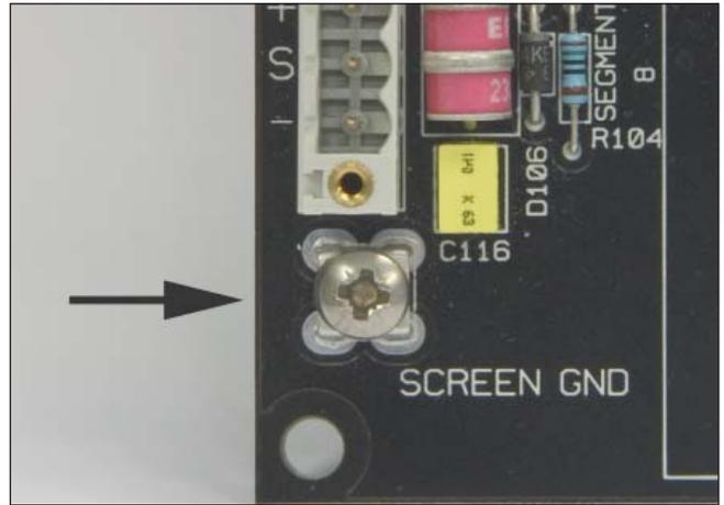
Figure 5.6 - Fieldbus segment screen ground terminal
