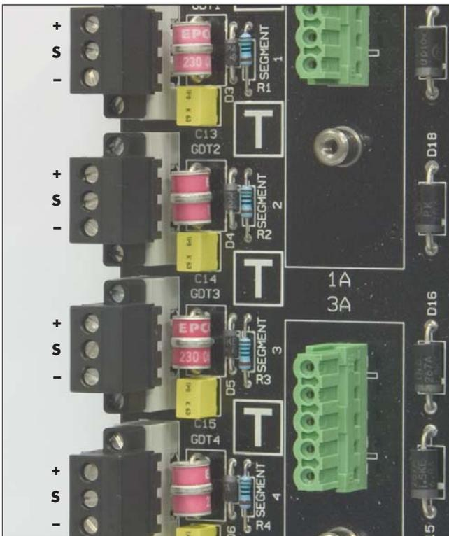
Figure 5.5 - Fieldbus segment connectors
