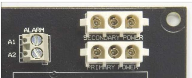
Figure 5.1 - Alarm and Power connections
