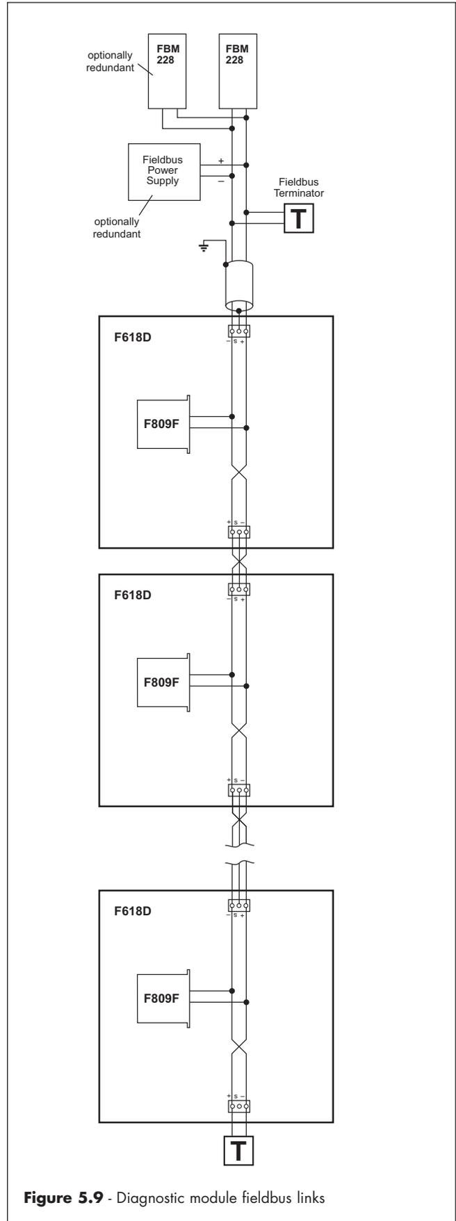
Figure 5.9 - Diagnostic module fieldbus links
