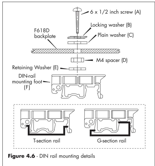
**Figure 4.6** - DIN rail mounting details
