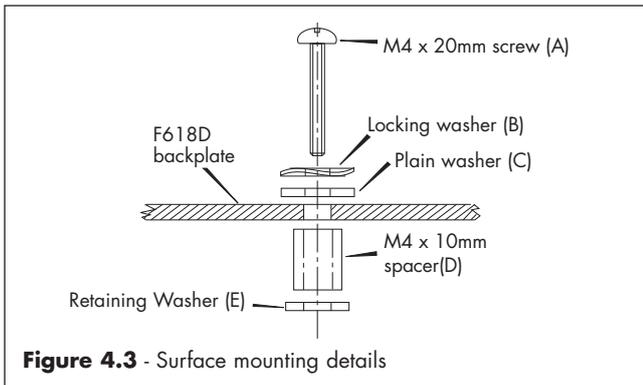
**Figure 4.3** - Surface mounting details
