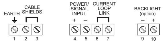
Figure 8 - MTL661/2/3/5 terminal connectors showing standard configuration and backlight options .
