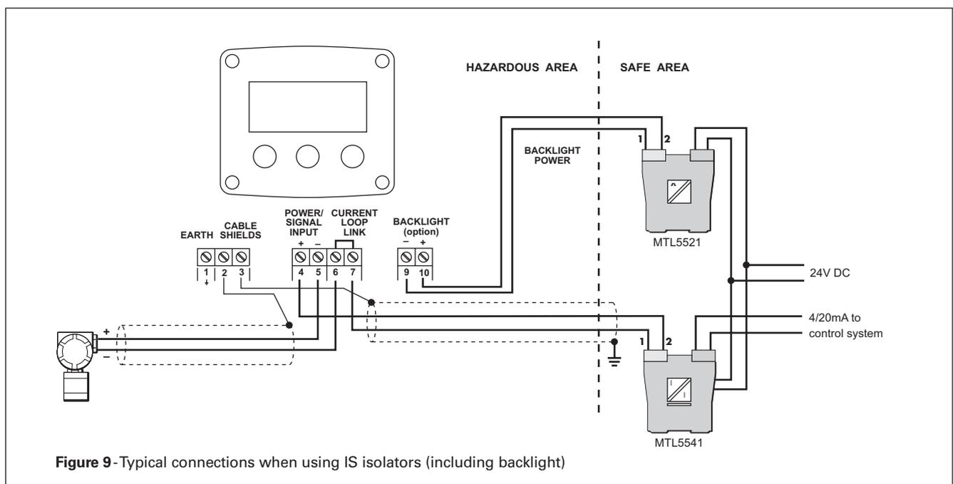
Figure 9 - Typical connections when using IS isolators (including backlight)
