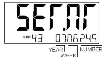
Figure 16: Display showing date and serial number
