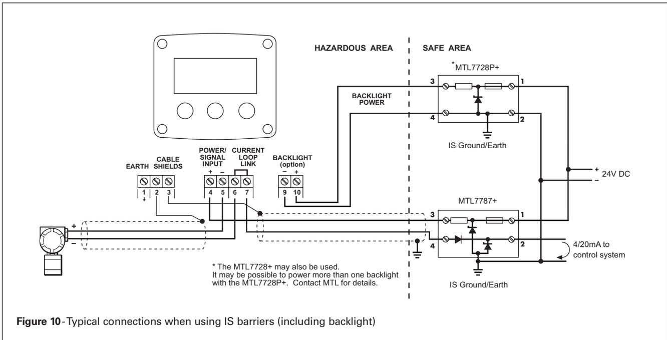
Figure 10- Typical connections when using IS barriers (including backlight)
