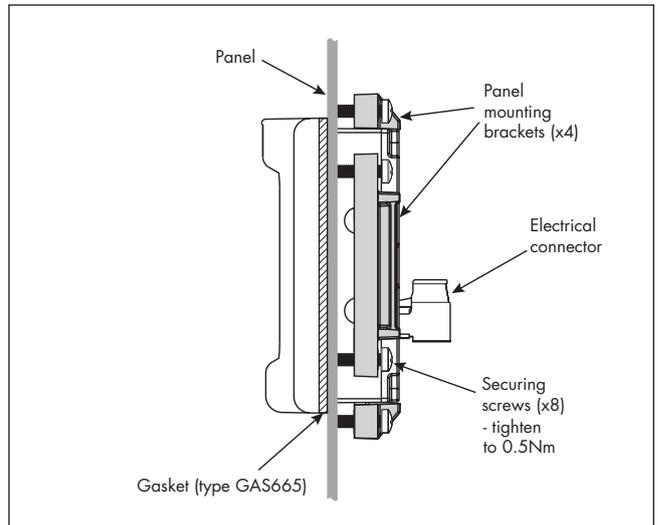
**Figure 18 Panel-mounting MTL665 display**
