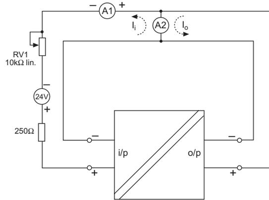
Figure 8.7: AI test circuit #3 "active i/p"
