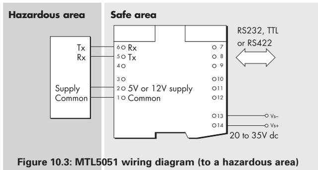
Figure 10.3: MTL5051 wiring diagram (to a hazardous area)
