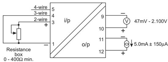
Figure 8.10: AI test circuit #5 “Resistance input”
