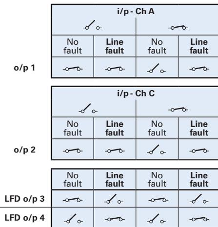
**Mode 12:** 3 ch with common LFD output
