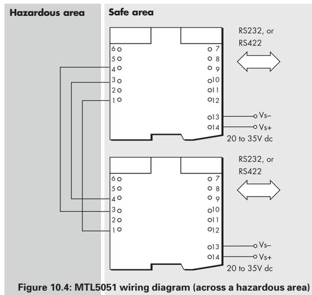
Figure 10.4: MTL5051 wiring diagram (across a hazardous area)
