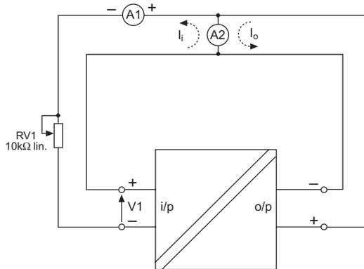
Figure 8.5: AI test circuit #1
