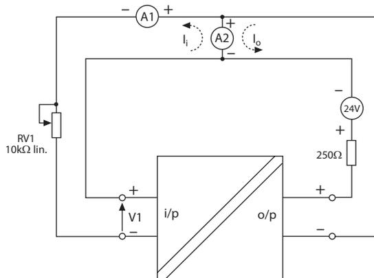
Figure 8.6: AI test circuit #2 “o/p sinking”
