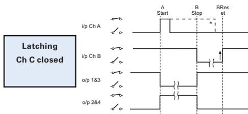
\* i/p Ch A can be open or closed when i/p Ch B opens to stop latch
