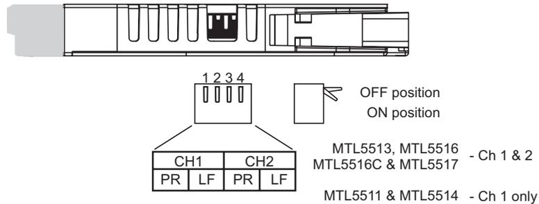
**Figure 6.1: Switches to set LFD and phase reversal**
