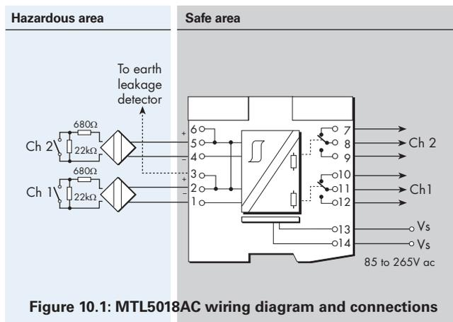
Figure 10.1: MTL5018AC wiring diagram and connections
