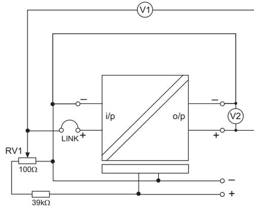
Figure 8.9: AI test circuit #5 “mV input”
