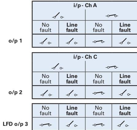
**Mode 10:** As mode 9 with line fault c/o
