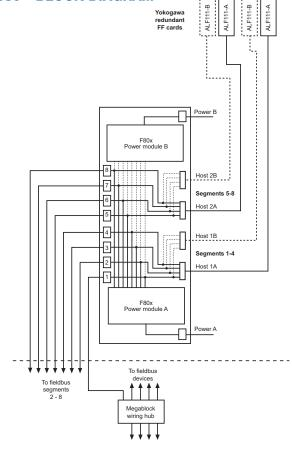
The above diagram shows a block diagram of how the F880 is wired. Note that the Chassis Ground and Alarm connection are not shown. The Diagnostic module is also not shown (see the F809F product specification). For detailed wiring information see the Installation Instructions for the F880 (Document number 502-089).
