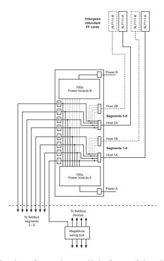
The above diagram shows a block diagram of how the F880-CA-RT is wired. Note that the Chassis Ground and Alarm connection are not shown. The Diagnostic module is also not shown (see the F809F product specification).
