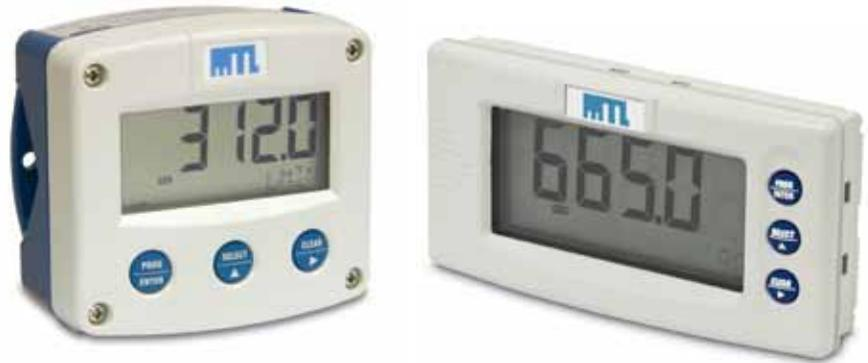
The **MTL661, MTL662, MTL663 and MTL665 digital indicators** enable process variables to be displayed locally in hazardous and general purpose plant areas. A typical example would be the re-transmission of mass/flow computations from the safe area, through a suitable MTL IS interface to the indicator in the hazardous area.
