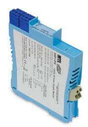
The 9491-PS Power Supply is the preferred method for supplying the 9460-ET series of intrinsically safe Ethernet modules and is based on an isolating power supply. It takes a 24V DC safe area / Zone 2 / Division 2 supply and produces an intrinsically safe, 12V DC nominal output capable of powering the Ethernet modules mounted in a Zone 1/ Division 1 hazardous area. The 9491-PS may be mounted in a safe area, Zone 2 or Division 2 hazardous area.
