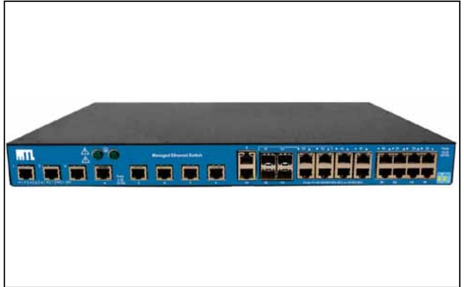
The MTL 9226/32-ETZ is an industrial Ethernet switch offering 26/32 total Ethernet ports including up to 8 super fast Gigabit ports and up to 4 noise-immune fiber optic ports. Its rugged and compact 1U case fits into standard EIA, WECCO and ETSI racks from 19" to 24"
