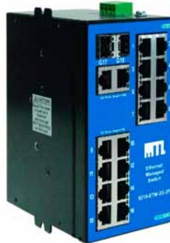
The 9218-ETM-2G-2F is an 18 port industrial Ethernet managed switch with 16 fast and 2 Gigabit combination ports that support both copper and fibre optic connections. This switch is designed to be rugged, reliable, real-time and secure. It combines compact DIN rail packaging, protected circuitry and powerful software to keep your system going even under the toughest conditions.
